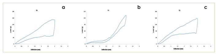
Fig 6. Load-deflection curves of multi-strand Ni-Ti (Supercable) wire at TO (a), T1 (b) and T2 (c) conditions.
