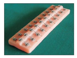
Fig 2. An acrylic plate for holding wire specimens in deflected state.
